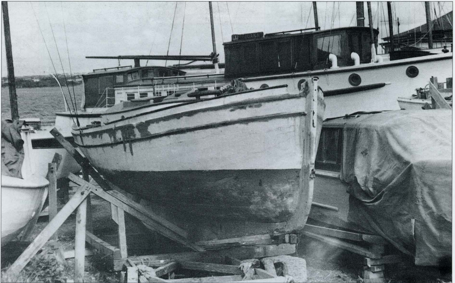
The first winter's refit at the Devonport Yacht Club, showing deep-bodied and slack-bilged hull with fore-keel rising to a deep forefoot.
